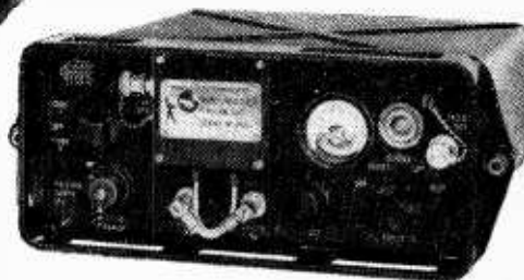
Below, Tactical navigation beacon MR 343 made by Rank Bush Murphy, incorporating a u.h.f. homer facility.
